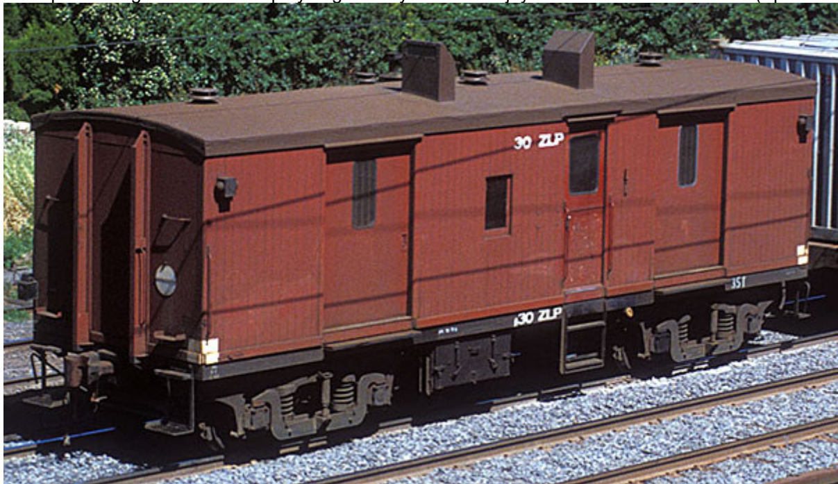
Photo 1 ZLP 30 note the white-painted brake indicator squares. Photo courtesy of Peter Vincent
