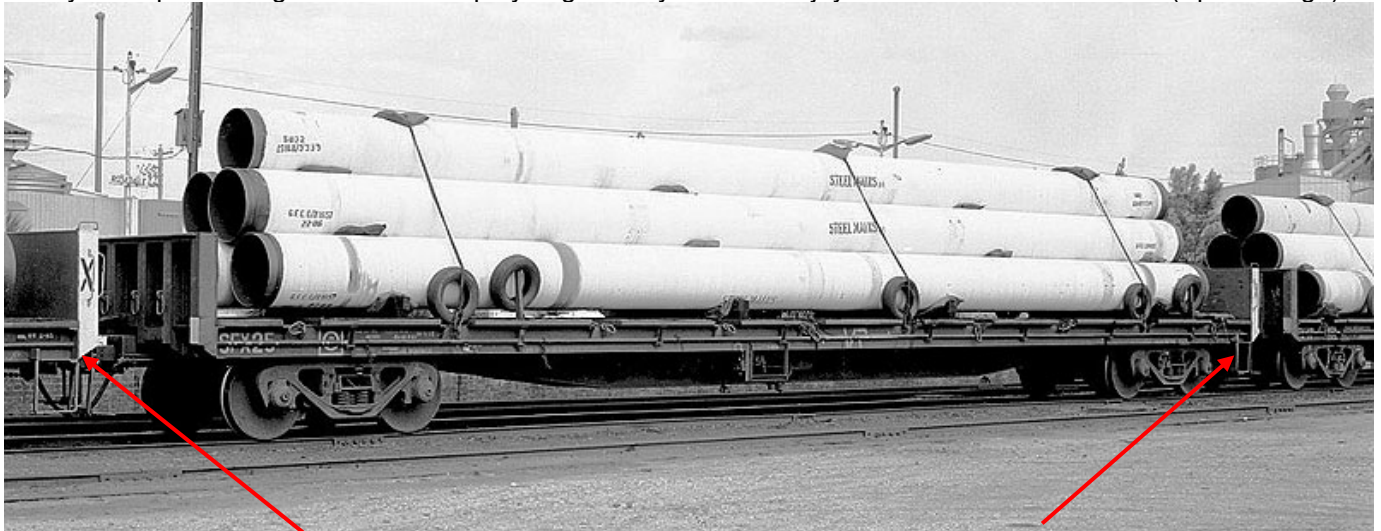
SFX-25 loaded with pipes. Note the white handbrake identification stripe on the bulkhead. Courtesy Rob O'Regan.
