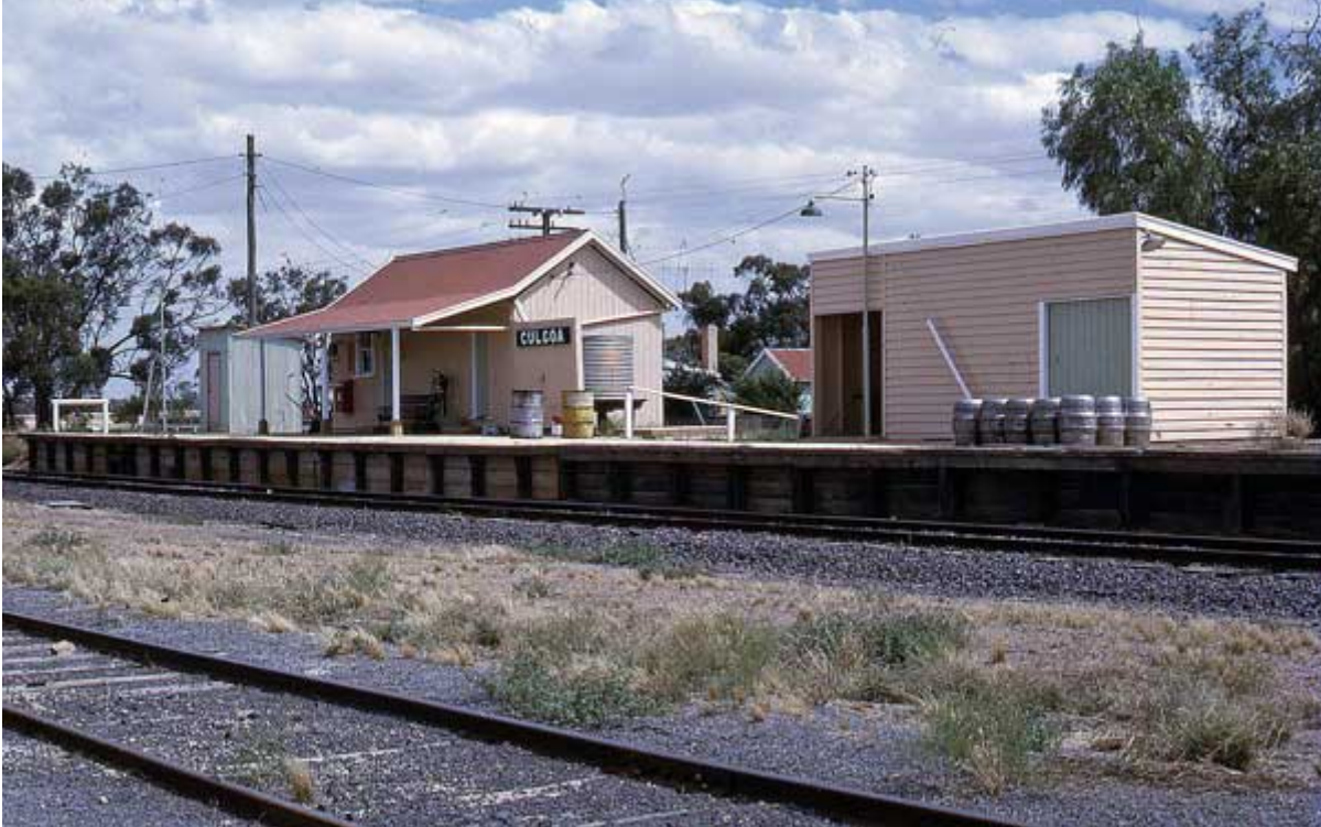
Typical VR 20ft portable station at Culgoa. It appears to be painted in the Mocha style. Note the extra detail around the portable and that the platform is both cement and wooden varieties. Photo courtesy of Neville Gee Collection.
