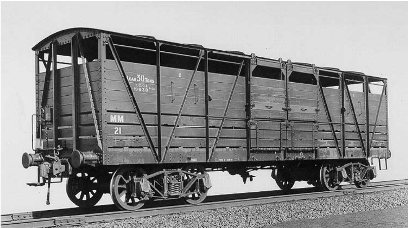
MM 21 as originally built at Newport workshops. Note the diamond frame bogies.
