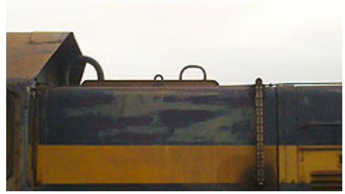
Fuel tank top side view. Photo courtesy Dave Crowhurst
