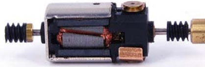
The altered motor fitted with a brass nut as a dampener
