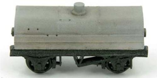
**Note wash the casting in warm soap water before gluing to remove the moulding release agent.** Glue the tank centrally using Selleys Kwik Grip to the underframe and trim the underframe to the length of the tank.
