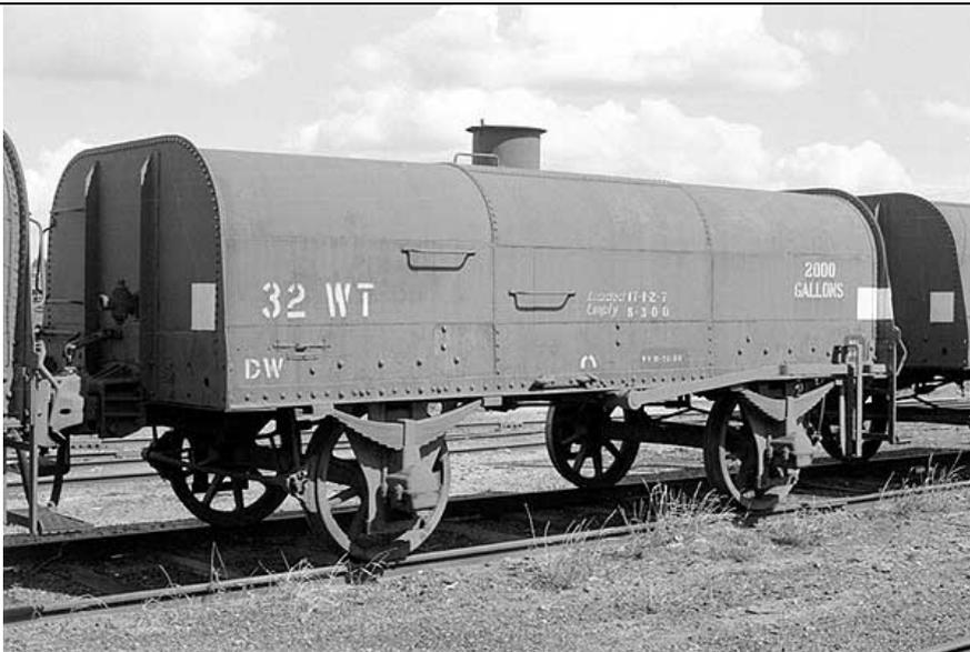
A typical WT no 32 is coupled to other units and is supplying Domestic Water. Note the small-stencilled 'DW', this indicated that the water was also available for drinking and as such the filler lids were always padlocked for safety.
