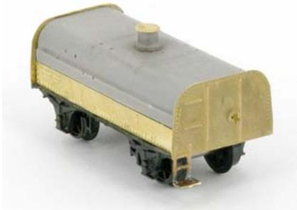
Glue the side brace etch to both sides as per this photo and after drilling a small hole into the casting for the tap at both ends glue the taps into the holes. Also, glue the filler hatch to the top of the tank.
