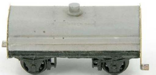
Fold up the shunter steps 90 degrees and solder at the corners or apply superglue sparingly. Glue the brass tank ends which include the shunter step to the casting ends and underframe. **Make sure that the etch sits above the physical tank by about 1/2 mm and has an even overhang at each side.** See photos of the prototype for clarity.
