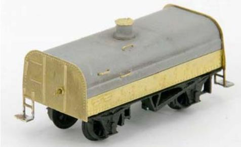
Fit handrails after drilling the pilot hole a bit deeper with a very fine drill bit. The fine brass wire should be bent to match the holes in the casting. Six are required all up. Glue the 30thou styrene pieces to the underside where the couplers will go. The model is now ready for painting, decaling and weathering.
