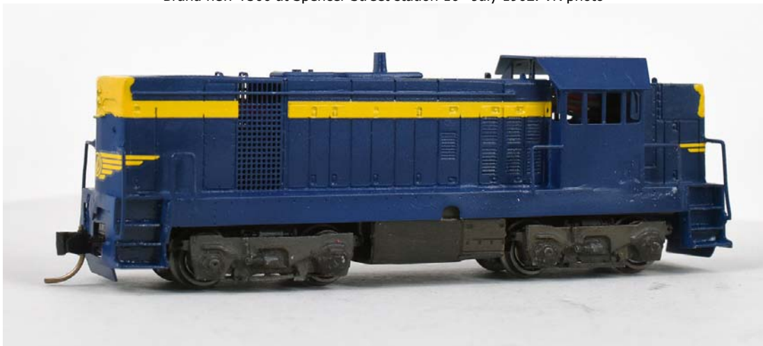
Finished model before glazing, cab number plates and marker lights. Note roof is not glued down yet and is only resting in place for the photo. I weather all my locos so this one will get the usual weathering details
