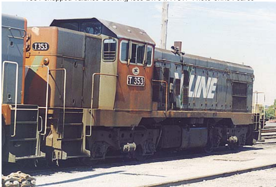
T 353 between duties at Geelong 04/03/1989. Note the different chopped valance compared to T351. Photo Chris Pearce
