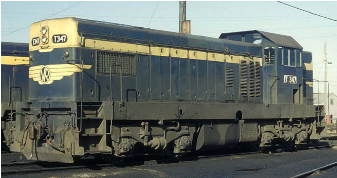
T347 staff exchanger cutouts and no cab valances, circa 1980. Photo courtesy of Mau Bau's website
