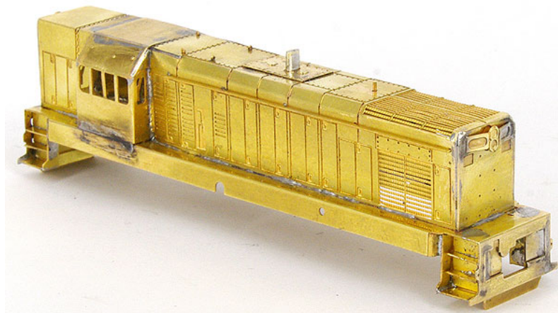
T333 takes shape after solder cleanup
