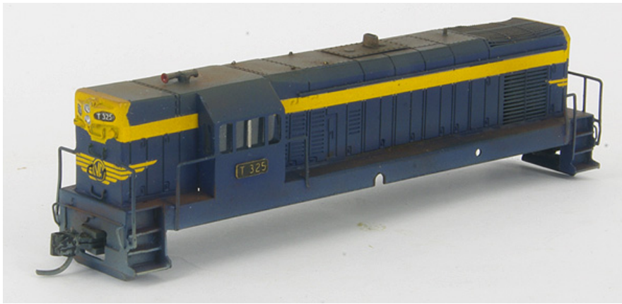
T325 has been lightly weathered using an airbrush and powders before being fitted with the mechanism
