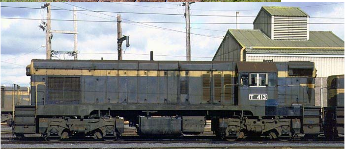
T413 dynamic brake fitted T class and sister low nose rest at Dynon Loco. Note the chopped valance which it acquired later on in its life. Photo courtesy of Mark Bau's website. T413 is currently preserved with sister locos T320, T333, T334, T341, T342 and T345.
