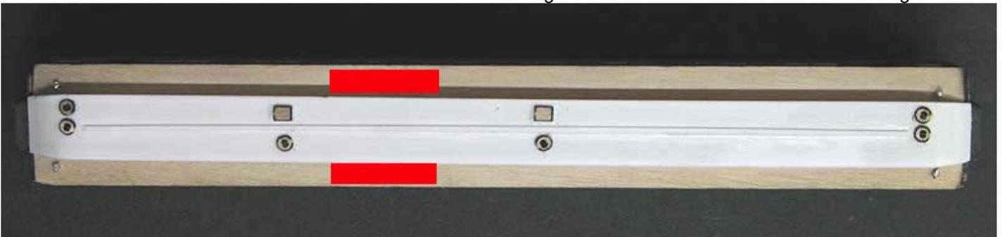
Completed roof before painting. Red indicates battery box location in the underframe in relation to roof orientation.
