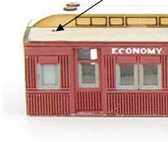
23. Cut the support leg and then glue the round water hatches (P15) and the small square roof hatches (P16) onto the outlines of the styrene roof (P12). Normal styrene glue will also do the job as it melts and bonds the timber to the styrene
