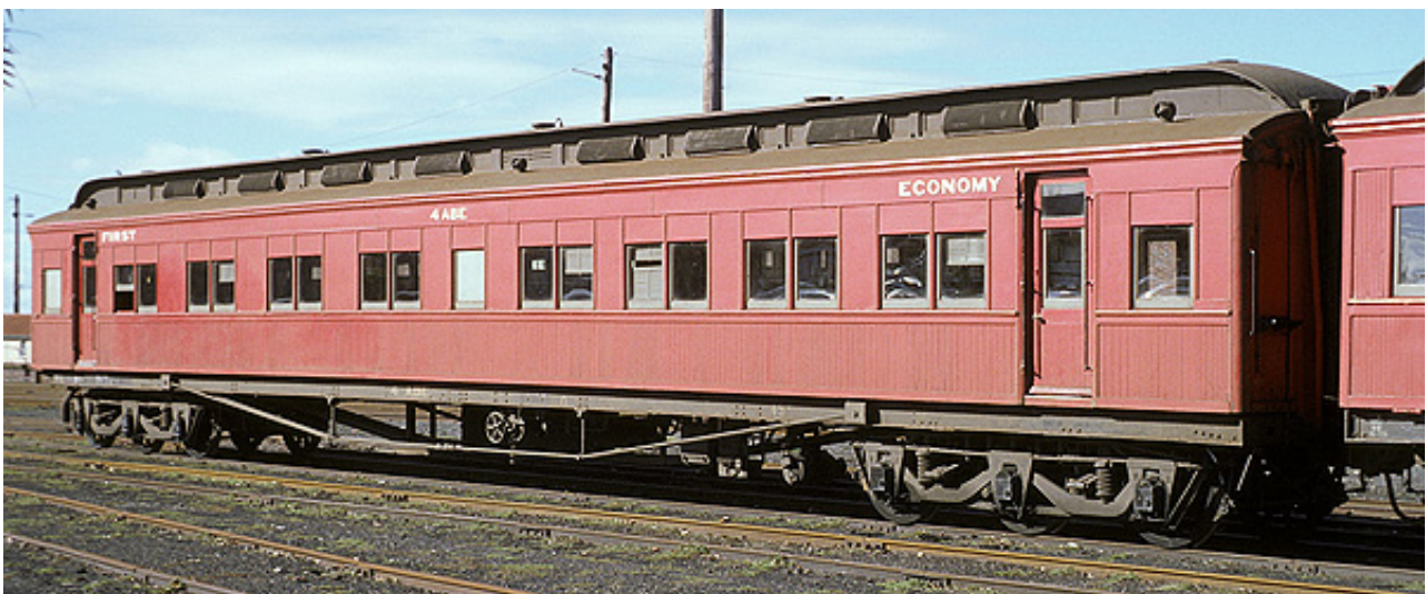
4 ABE Courtesy of Geoff Winkler – Note the two painted out windows of the toilets.
